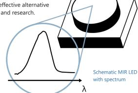
Any **custom wavelength** is possible: You tell us what you need and we deliver it. With our outstanding technology we design any wavelength **between 2800 nm and 6500 nm** within a spectral window where your desired emission wavelength reaches at least 95% of the maximum spectral intensity.
